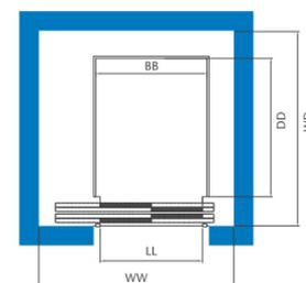
WW - Well Width; WD- Well Depth; BB - Car Width; DD - Car Depth; LL - Door Opening
